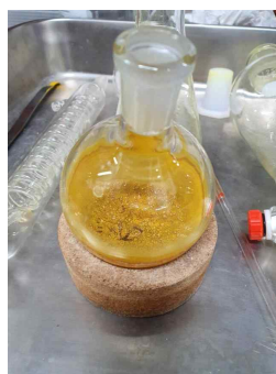
Figure 15. Final product (4-amino-3-nitrobenzoic acid methyl ester)
