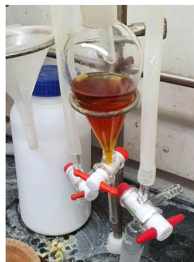
Figure 10. Add 20 mL of ethyl acetate to the funnel.
